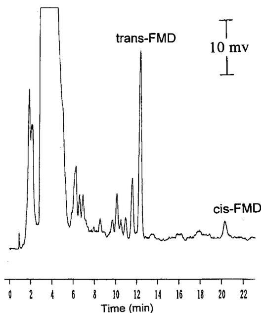
**Figure 2.** Chromatogram of methanol extract of *A. bidentata*. *cis*-FMD: *N-cis*-feruloyl 3-methyldopamine; *trans*-FMD: *N-trans*-feruloyl 3-methyldopamine. HPLC conditions, column: Inertsil ODS-P, 5  $\mu\text{m}$ , 25 cm  $\times$  4.6 mm I.D.; mobile phase: A-B (A = acetonitrile; B = water), 0 min, 25 : 75, 14 min, 30 : 70 and 30 min, 35 : 65; flow rate: 1.0 mL/min; detection wavelength: 300 nm.
